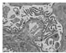
Specimen: ultra thin section of mouse kidney (contrast reversion) Accelerating voltage: 5.0 kV Scan speed: 0.04 usec/pixel (5,120 × 3,840)
